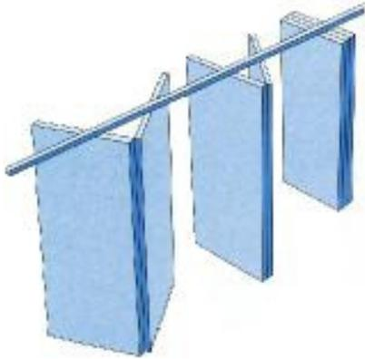
**Centre Stacking Individual Panel** - Individual, single panel system. Panels are parked at the end of the run of track when the wall is open. The panel has a single carrier. The system is best utilized in areas where the centre stacking of panels might be the most feasible and practical option for parking of the panels and when parking of panels of the main track is not a possibility.
